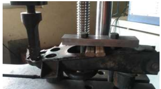
Fig. 3.8 Testing wishbone arm on UTM
