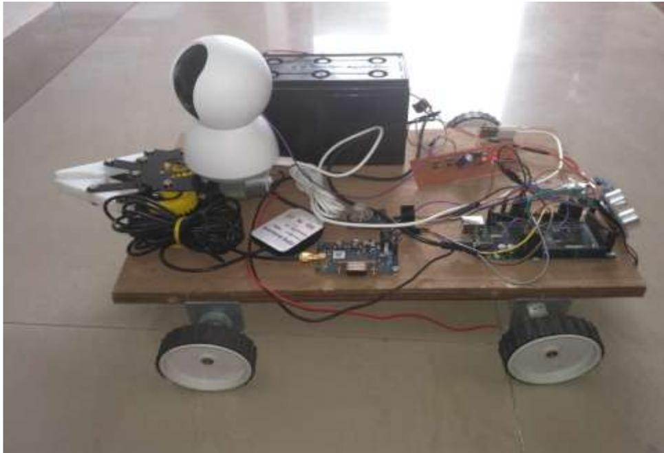
**Fig 6: Dual Arm Tele-Robotic System Hardware**
