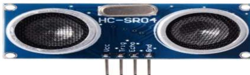
**Fig 5: Ultrasonic sensor**
