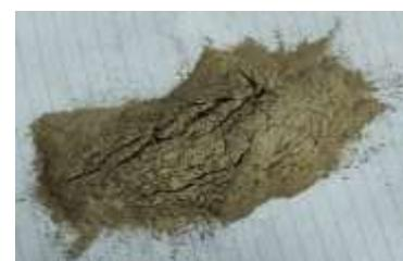
**Fig 1: Untreated Bagasse Ash**
