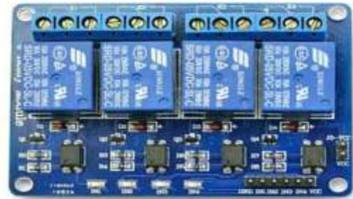
**Fig -4:** 4-Channel Relay Module
