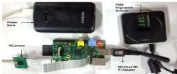
Fig -6: Basic Hardware setup of RPi
