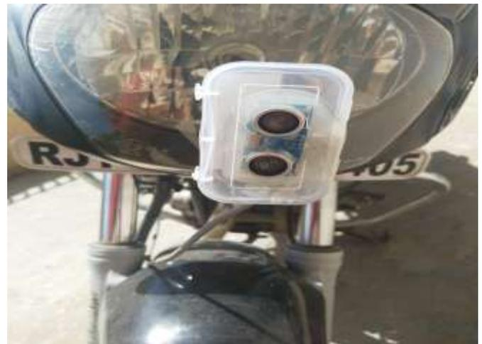
Fig-1. Ultrasonic Emitter and Receiver Mounted on Motor Bike
