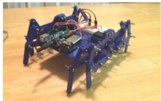
Figure:- A typical Swarm robot working on klann mechanism
