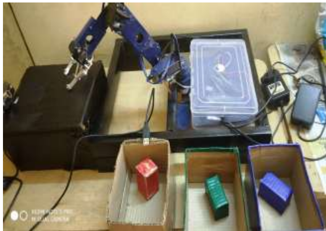
Figure-12: Experimental Setup of Pick and Place robot
