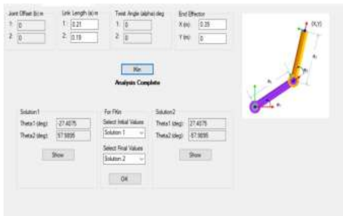
Figure-10: Angle determination using Robo-Analyzer
