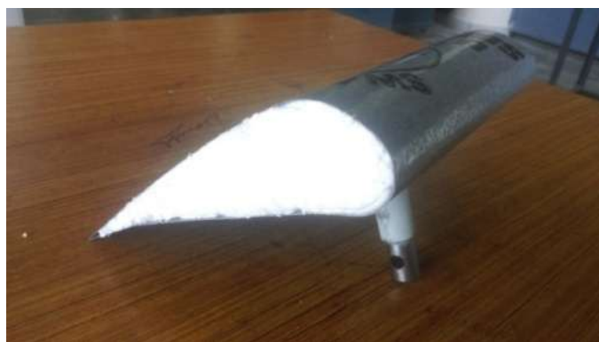
Fig -4: Fabricated spoiler with fixture attachment
