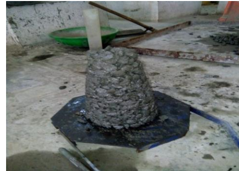
Fig 4.1 Slump cone Test
