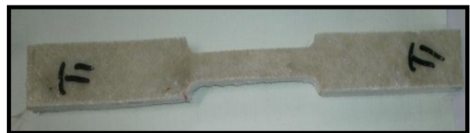
Fig-3: Specimen before Tensile Testing
