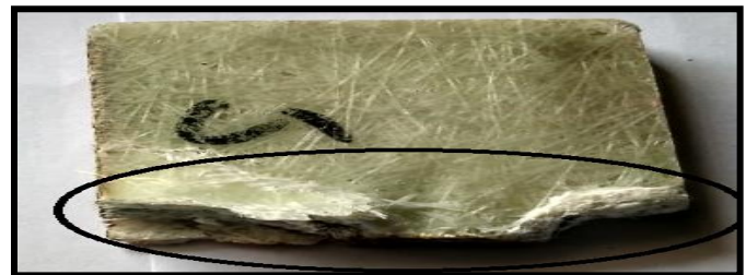
Fig-7: Specimen after Compression Testing
