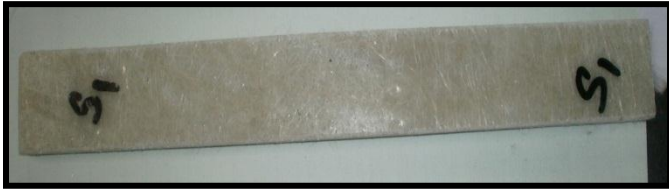
Fig-14: Specimen before Shear Testing
