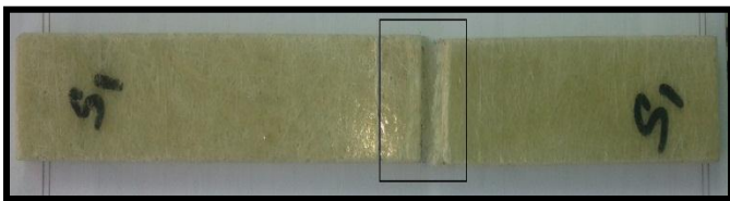
Fig-15: Specimen after Shear Testing
