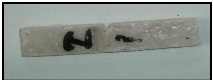
Fig-12: Specimen before Impact Testing
