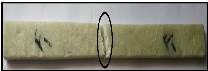
Fig-10: Specimen after Flexural Testing
