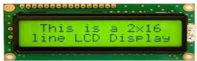
**LCD** (Liquid Crystal Display) screen is an electronic display module and find a wide range of applications. A 16x2 LCD display is very basic module and is very commonly used in various devices and circuits. These modules are preferred over seven segments and other multi segment LEDs. The reasons being: LCDs are economical; easily programmable; have no limitation of displaying special & even custom characters (unlike in seven segments), animations and so on.
