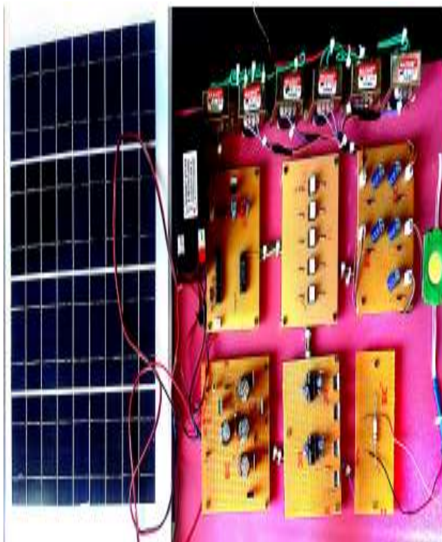
Fig-12: Hardware Setup for Seven Level inverter
