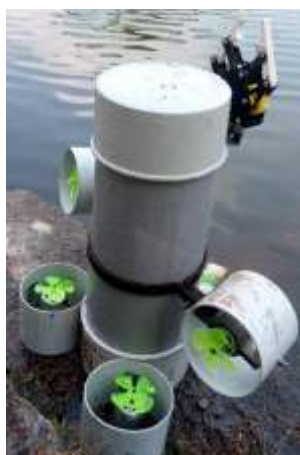
Fig -8: Finalized structure with thrusters and arm
