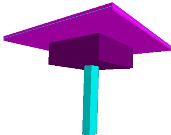
Fig. 2: Flat Slab with Drop
