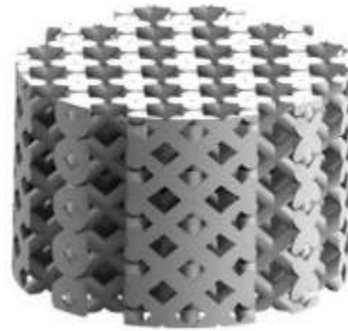
Fig 1.1.2 Crosssectional strut structure
