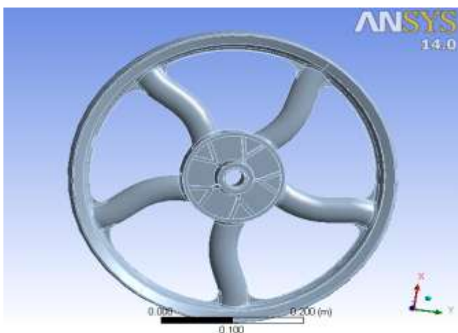
Fig-10: Modified 3D design of alloy wheel
