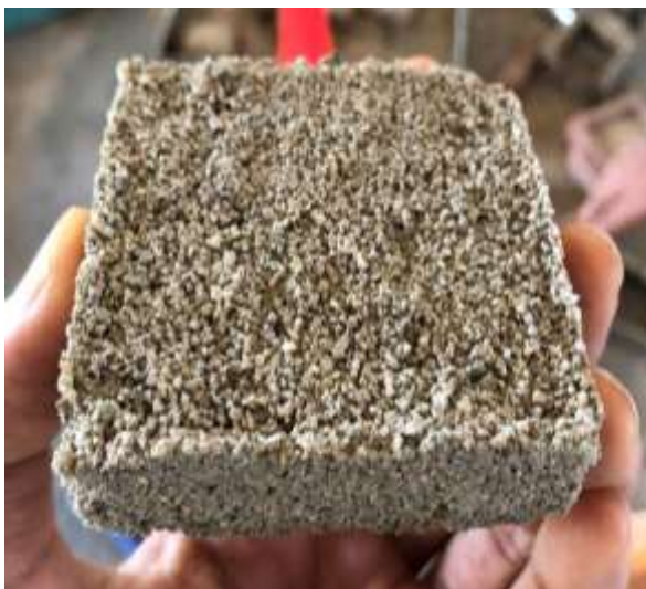
Fig -1: Grouted specimen for direct shear test
