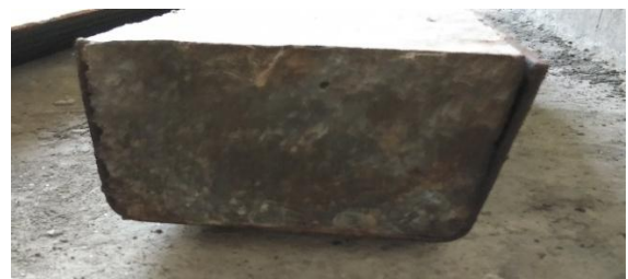
Fig-5: Failure of rectangular CSCC beam (side view)
