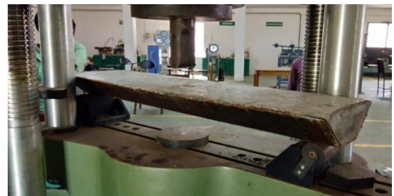
Fig-6: Failure of trapezoidal CSCC beam
