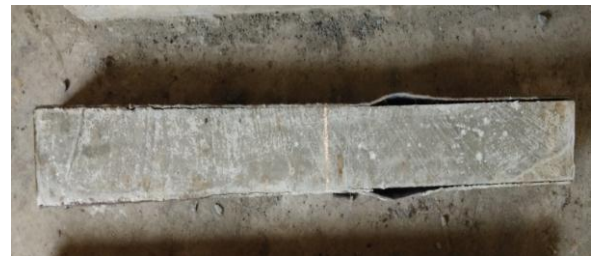
Fig-4: Failure of rectangular CSCC beam (top view)
