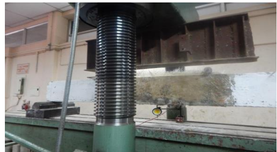
Fig -3: Testing of U wrapped specimen (U3)
