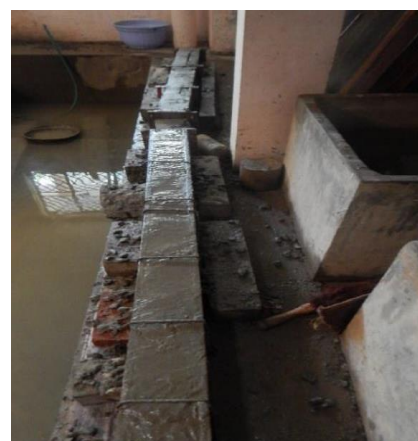
Fig -1: Reinforced concrete beam specimen
