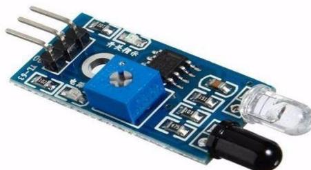
Infrared Sensor Module has built-in IR transmitter and IR receiver that sends out IR rays and looks for reflected IR rays to detect presence of any obstacle in front of the sensor module. The module has on board potentiometer that lets user adjust detection range. The sensor has very good and stable response even in ambient light or in complete darkness.
