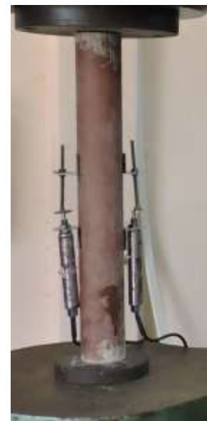
Fig -2: LVDT fixed on the specimen for measuring vertical strain
