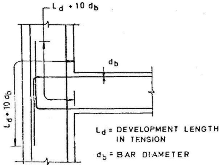
Fig. 1.1 Anchorage of beam bar in an external joint
