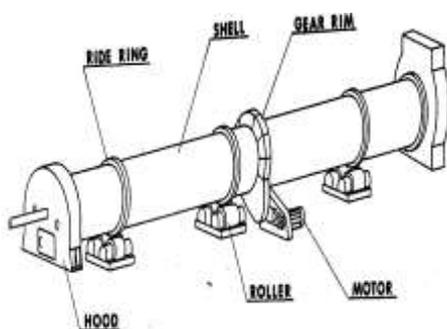
Fig.2 Construction of Calcination Drum.
