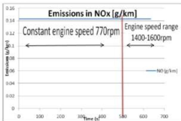
Figure 3: Nitrogen Oxide Emissions of Standstill Testing
