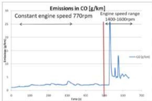
Figure 2: Carbon Monoxide Emissions of Standstill Testing
