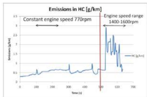
Figure 1: Hydrocarbons Emissions of Standstill Testing
