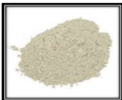
Fig -2: Powdered Bentonite Clay
