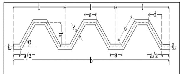
Fig -1: Cross-section of corrugated plate and its dimension
