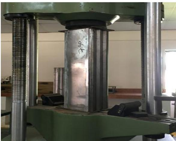
Fig -1: Test-setup of column
