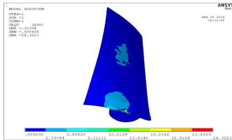
Figure 9 Blade Von Mises stress
