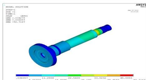
Figure 10 Shaft Von Mises Stress
