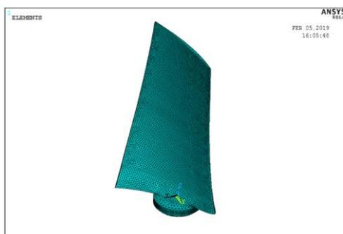
**Figure 6 Meshing of Fan Blade**
