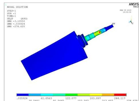
Figure 11 Assembly Von Misses Stress
