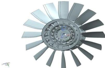
**Figure 5 Final Assembly of Axial Fan Rotor**
