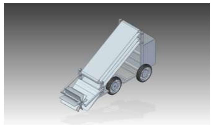
Fig 6.2: 3D Structure of waste collecting machine
