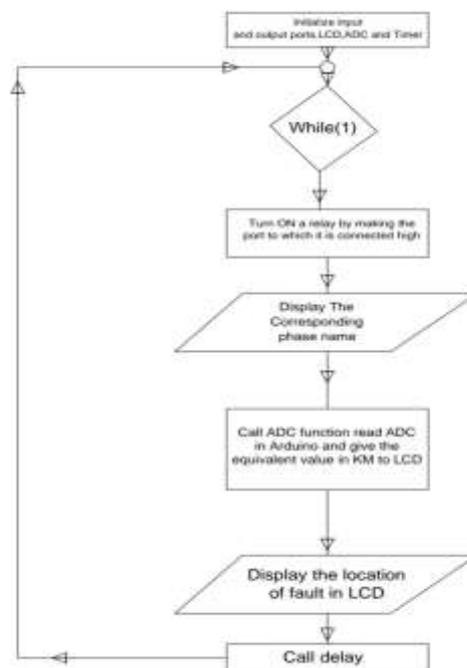
fig-2: block diagram of flow chart
