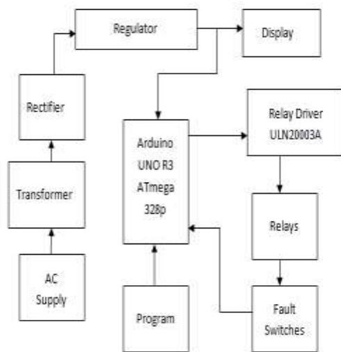
fig-2: Circuit diagram of system
