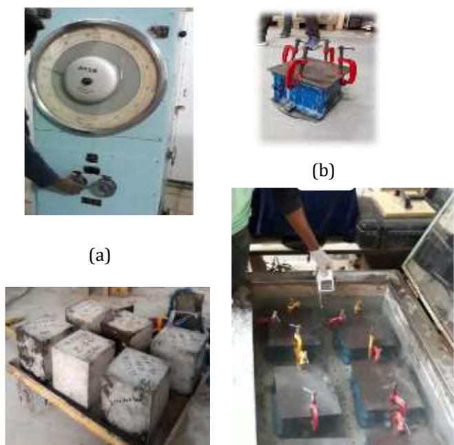
**Fig - 1:** Hydraulic CTM (a), Mold for accelerated curing (b), Specimens immersed into warm water (c), Accelerated curing tank (d) and accelerated curing cubes ready for compressive strength test (e).
