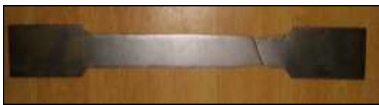
Fig -2: Tensile test specimen after testing
