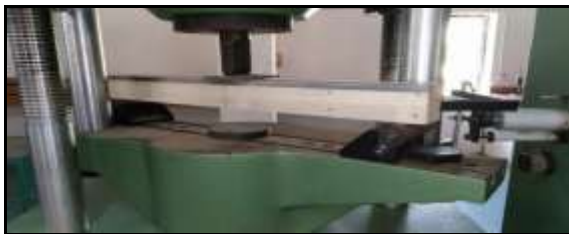
Fig -3: Test set up of the composite beam using Z section
