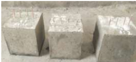
Fig. -1: Conductive Concrete Specimen
