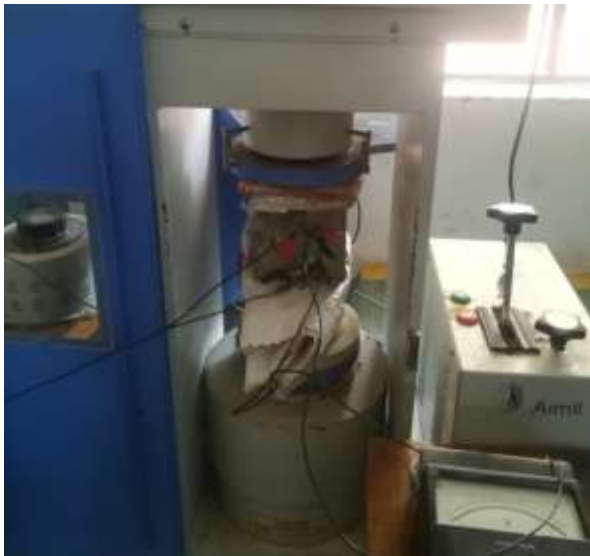
Fig. -4: Resistance measurement on a typical specimen
