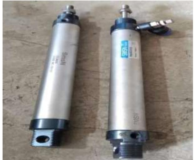
Fig -2: Pneumatic Cylinders
