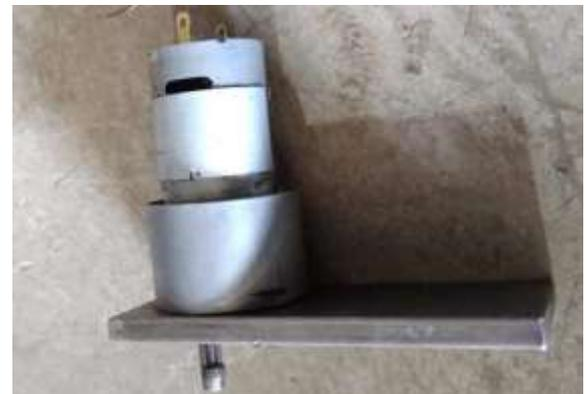
**Fig -5:** DC Gear Motor
