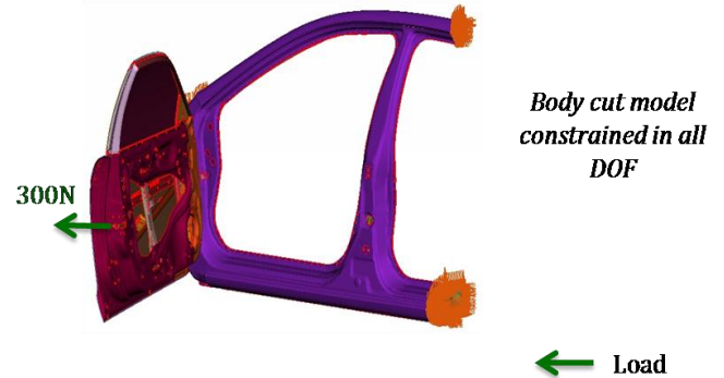
Fig -6: Static Over Check model setup
