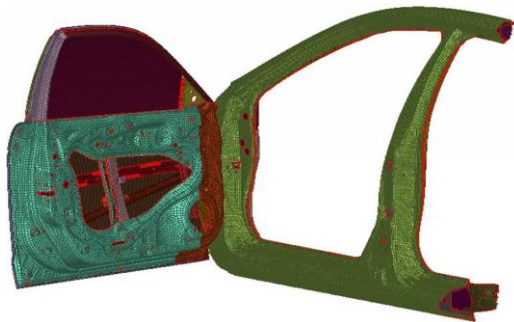
Fig -4: Finite Element Model of Front Door Assembly
