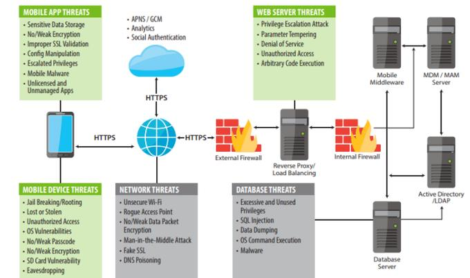
Fig.1 Data secure in Mobile Application
