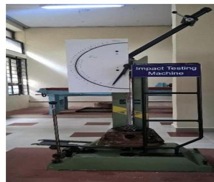
Figure 6. Impact testing of the specimen
