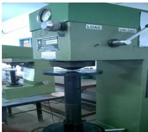
Figure 7. Hardness testing of the specimen
