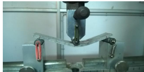
Figure 4. Flexural testing of the specimen.
