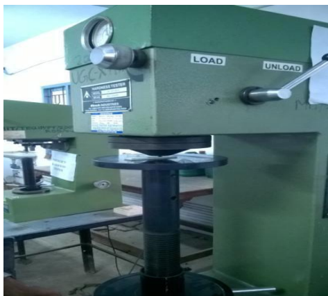
Figure 7. Hardness testing of the specimen
