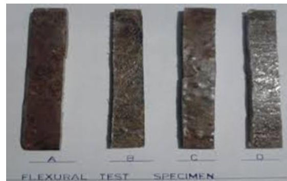
Figure 9. SBCCC hybrid after flexural test
