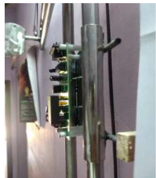
Fig - 10 Side view of the RFID reader attached to the gantry head
