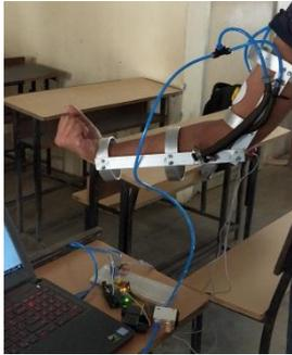
Fig .5 Assembly of pneumatic arm
