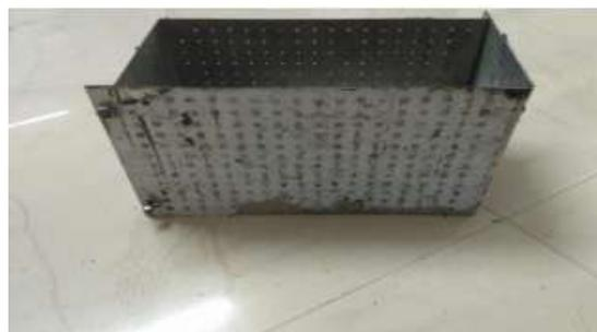
**Figure 4.** Mould for masonry block
