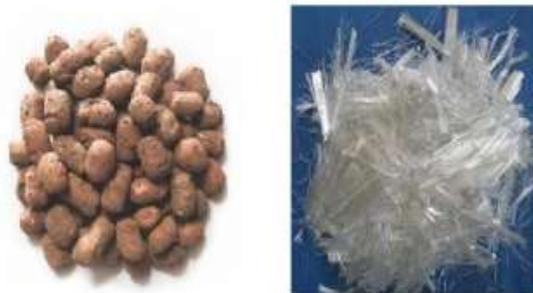
**Figure 2:** Expanded clay aggregate and glass fibre
