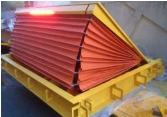
Fig Side View of Crash Barrier.
