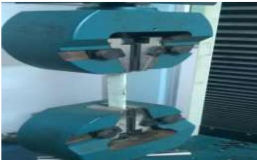
Figure 5. Tensile testing of the specimen.
