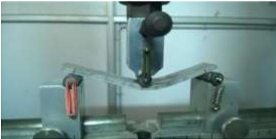
Figure 4. Flexural testing of the specimen.
