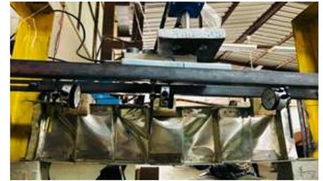
Fig -6: Arrangement of Dial Gauges and Beam loaded into the setup
