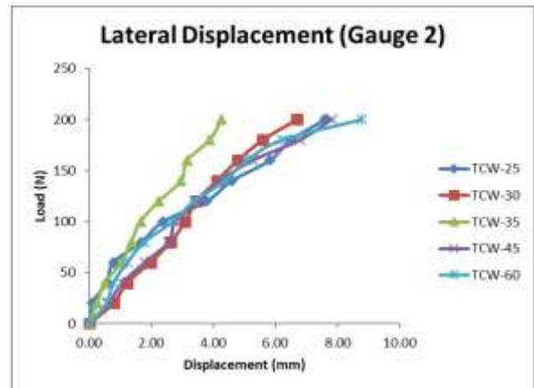
Graph -1: Load vs Lateral Displacement
