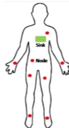
**Figure 2: WBAN Body Area Network with Eight Nodes**
