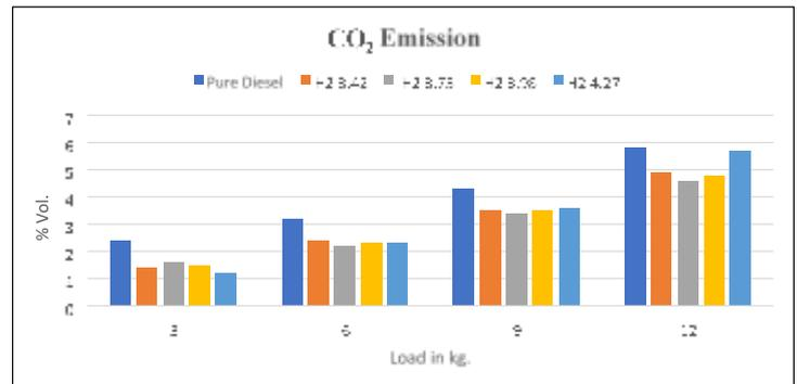
The variation in CO<sub>2</sub> emission is as shown in graph. It is observed that CO<sub>2</sub> is higher with diesel as compared to H<sub>2</sub>. With diesel CO<sub>2</sub> emission observed is 3.20% vol<sup>m</sup> when we introduced H<sub>2</sub> 3.75 ml/sec then in gives 2.2 % vol<sup>m</sup>. The most favorable outcome is of CO<sub>2</sub>, as it is the most domination gas for global warming and for climatic change. The CO<sub>2</sub> emission are less as compared to pure diesel engine.
