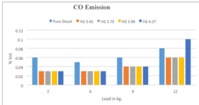
It is observed that CO is higher with diesel as compared to H<sub>2</sub>. With diesel CO emission observed is 0.06% vol. When we introduced H<sub>2</sub> then in gives 0.03 % vol. but under high applied load at 12 kg the output CO is more as compared to diesel engine. But the CO emission is reduced during load between 3 to 9 kg.
