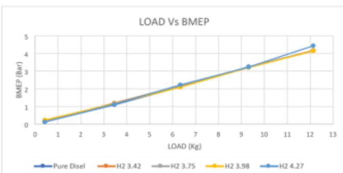
The experimental result shows the variation of break mean effective pressure (BMEP) with respect to load variation. It is observed that when we blend H<sub>2</sub> 3.98 ml/sec into diesel
