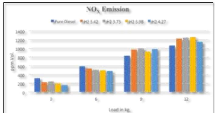
kg load pure diesel gives 587 ppm volm of NO<sub>x</sub> whereas when we introduces H<sub>2</sub> then it emits less NO<sub>x</sub>. At 3.75 ml/sec of H<sub>2</sub> it gives 507 ppm volm of NO<sub>x</sub>. The NO<sub>x</sub> emissions are within limit but when at maximum load is increased the emission of NO<sub>x</sub> are increased.
