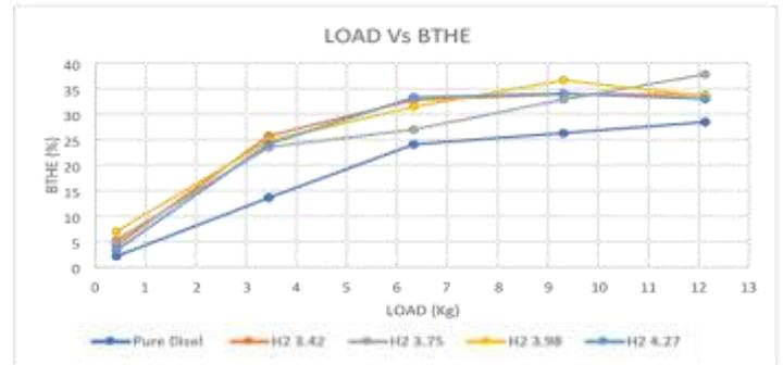
The experimental result shows the variation of break thermal efficiency (BTHE) with respect to load variation. It is observed that when we blend H<sub>2</sub> 3.98 ml/sec into diesel it increases the break thermal efficiency as it is produced by pure diesel.
