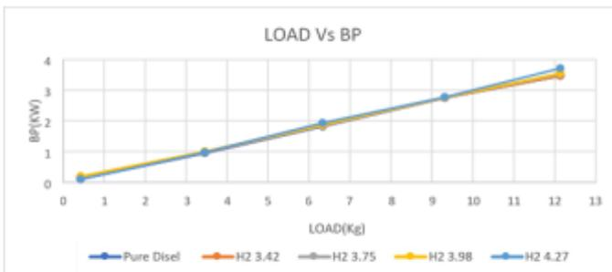
The experimental result shows the variation of Break Power with respect to load variation. It is observed that when we blend H<sub>2</sub> 3.98 ml/sec into diesel it produces same break power as it is produced by pure diesel.
