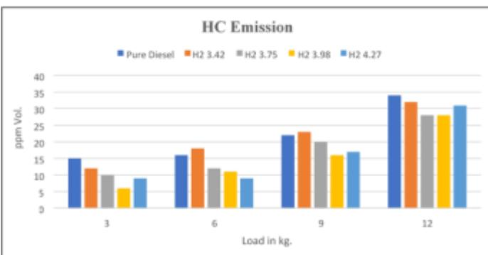
The graph shows variations in HC. It is observed that when we introduce H<sub>2</sub> more than 3.75 ml/sec it gives less HC emission than the pure diesel. At 6kg load pure diesel gives 16 ppm vol<sup>m</sup> of HC whereas for 3.75 ml/sec of H<sub>2</sub> it gives 12 ppm vol<sup>m</sup> of HC. The overall HC emission is halved and it is beneficial for any range of load as the HC emission during high load is also less than diesel.
