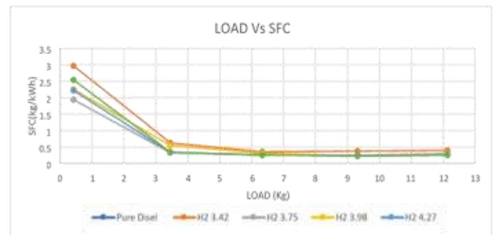
The experimental result shows the variation of specific fuel consumption with respect to load variation. It is observed that when we blend H<sub>2</sub> 3.98 ml/sec into diesel it decreases the specific fuel consumption as it is produced by pure diesel.
