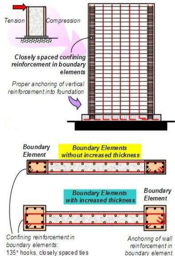
Fig -1: Building with Shear wall
