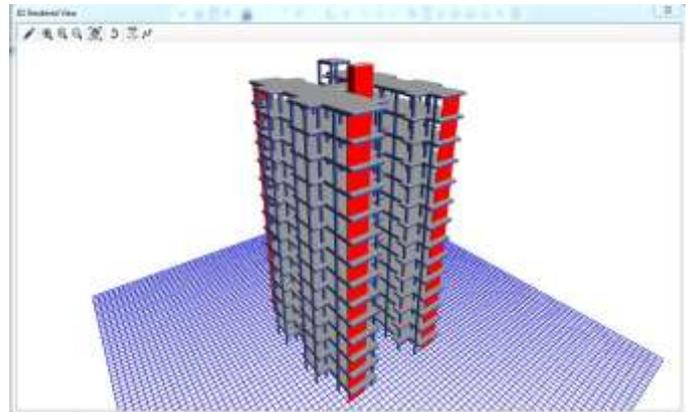
**Fig -4:** Building with Shear wall Having Opening.
