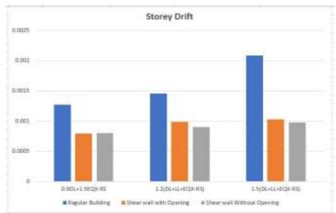
**Graph -2:** Graph of storey drift for regular structure, with shear wall and shear wall with opening structure.
