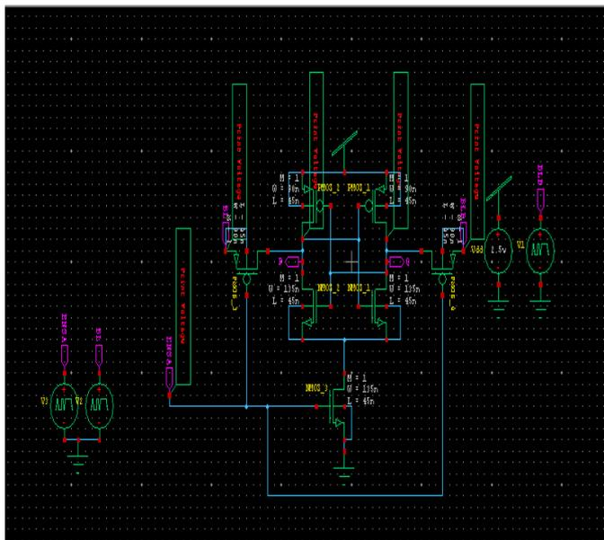
Fig -5: Schematic of Voltage Mode SA
