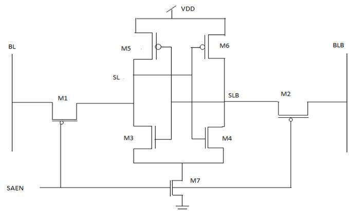
Fig -1: Cross-coupled voltage mode SA [4]
