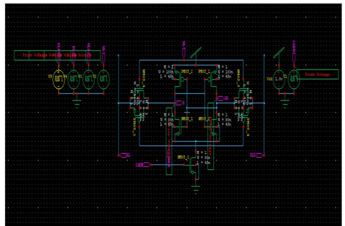
Fig -7: Schematic Diagram of Transmission Gate VMSA
