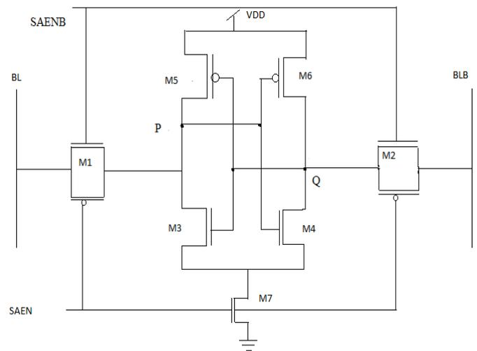
Fig -4: Transmission Gate VMSA [3]
