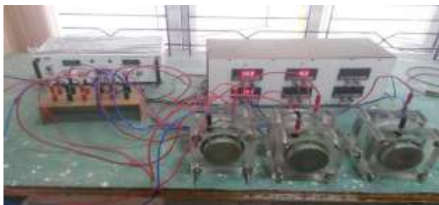
Fig-6: RCPT Test
