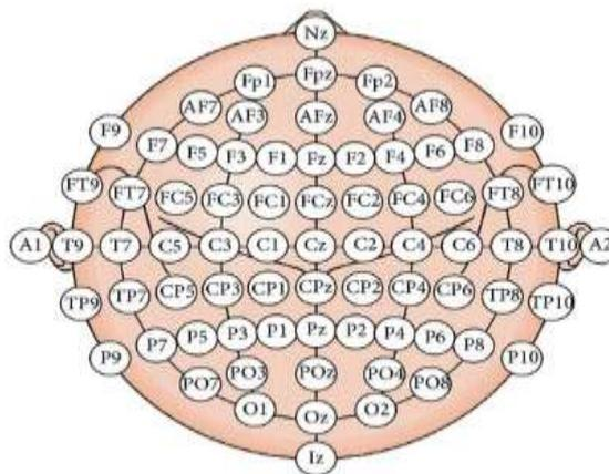
Fig -1: 10-20 electrode placement system [11]
